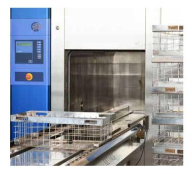
**Temperature and Pressure** As Temperature is directly linked to the lethality value, this parameter can also be used to check how well the autoclave performs. Additionally, when using Moist Heat Sterilizers, pressure can be converted into theoretical temperature which can then be compared to the actual temperature in order to evaluate if the steam is saturated. This eliminates the risk of air pockets, which could otherwise jeopardize the process.
